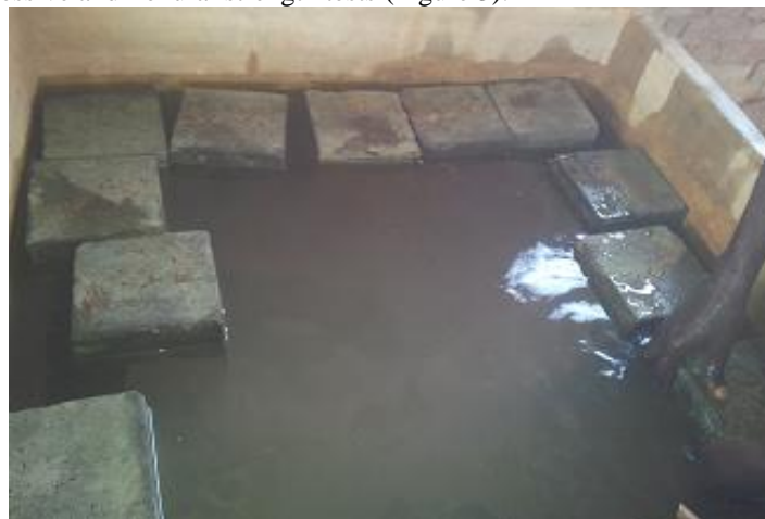
Figure 3: Curing Tank with the Concrete Specimen
