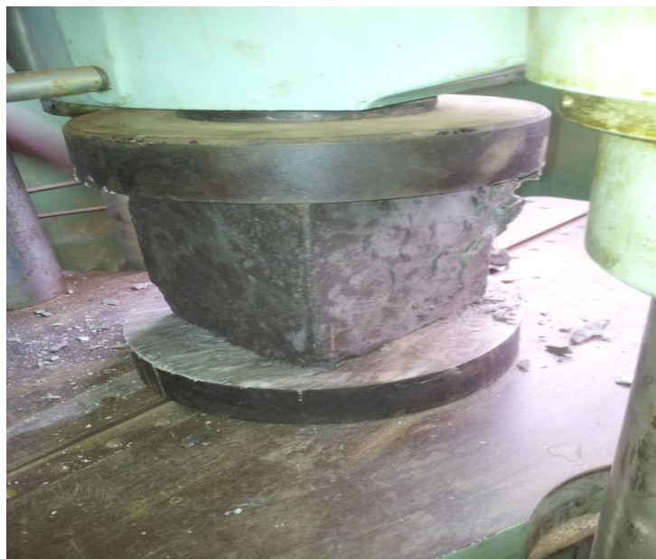
Figure 4a: Compressive Strength Test Using concrete cube specimen
