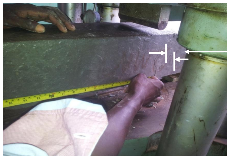
Figure 4c: Concrete Beam Specimen after Failure
