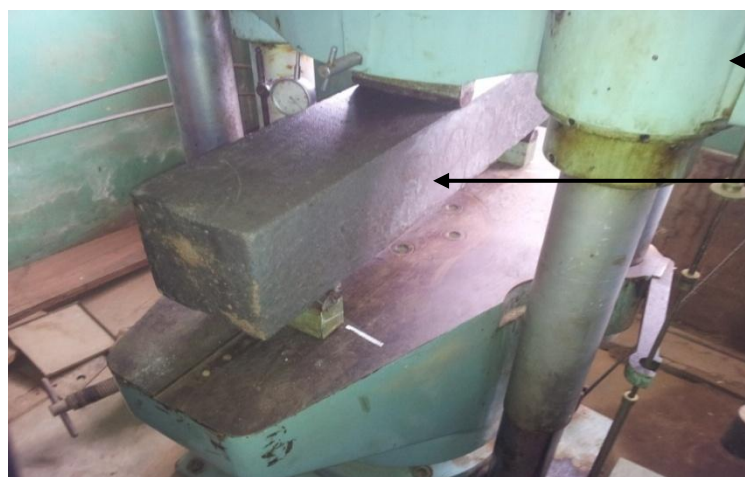
Figure 4b: Flexural Strength Test Using Concrete Beam Specimen (UTM: Avery-Denison EN76066 7113DCJ; Capacity of 600kN)
